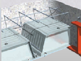
Shallow floor beam with deep composite deck
