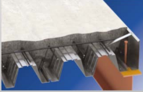
Downstand composite beam with composite shallow deck
